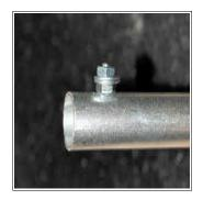
The aluminum dipole elements are separated and connected by a plastic rod which feels the inside of the aluminum tubes to prevent the saddle clamps from pinching or compressing (crushing) the aluminum tubes. It also serves as an insulated divider keeping the ends of the to tubular elements approximately 1 inch from each other.
