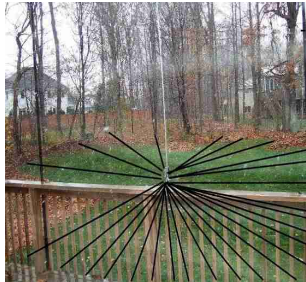
Graphic depicting approximate location of first 27 radials – 50 are planned.
