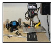
Two small holes are drilled approximately . 5" inch from the "center" ends of each element to accommodate a small  $6-32 \times 2$ " machine screw that is secured with a nut. Outside of that is a wing nut to attach the lugs on the leads from the 1:1 line isolation choke/balun.
