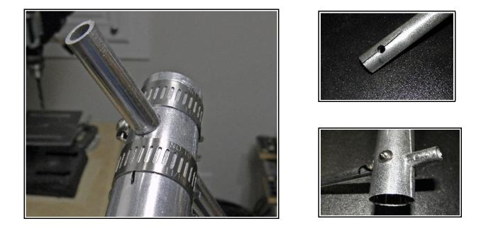
The ends of cut tubing were rounded off on a grinder to avoid injury-causing burrs, and all holes in the aluminum element-to-mast plate were all done on a moderately competent drill press.
