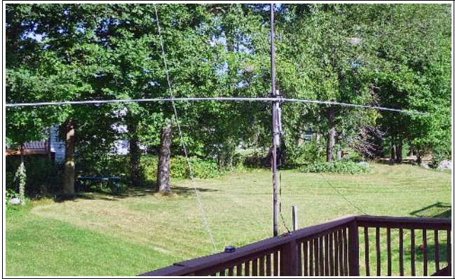
10 meter antenna temporarily set for initial tuning and adjustment above the rear deck.
